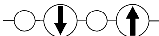
Figure 28. Schematic representation of the mean-field ground state of 1D extended Hubbard model with \Delta_d = 0 in the charge ordered state. The size of the circle and the arrows represent the charge density on each site and the spin moment, respectively.
